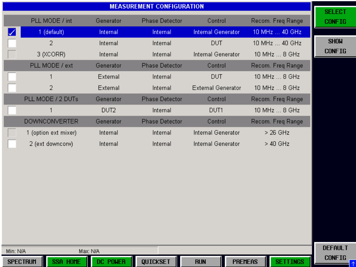
Fig. 5-4 MEASUREMENT CONFIGURATION dialog box
