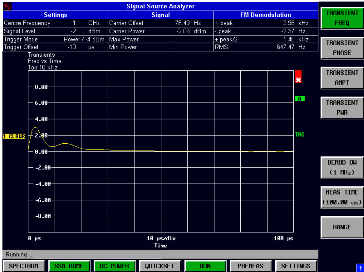
Fig. 5-24 Frequency settling of the generator
