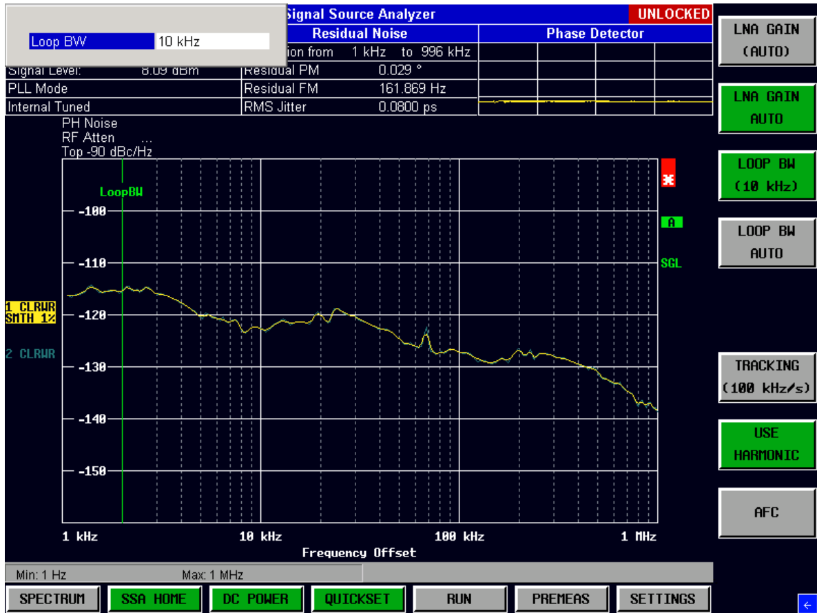
Fig. 5-16 Phase noise measurement result display
